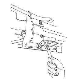
Install provided spacer (18) and M6 bolt (13) into upper mount as shown on both the Drive and Idler linkages. Do not tighten.
