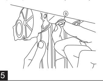
Slide mounting T-nut into position, Center board in rail pocket. Tighten fasteners to 10 ft-lbs.
