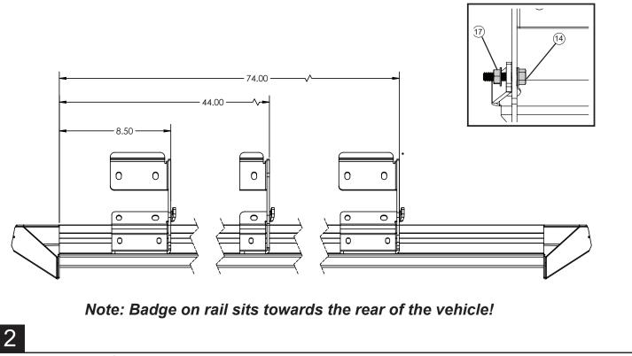
Set rail up into position. Starting with the rear bracket work towards the two front brackets. Slide Brackets over captive studs and use provided Nuts 8x (10). Snug to body and torque to 16 ft-lbs.
